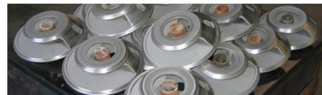
performance of the valve, requiring routine replacement of both the stationary and rotating valves. EIC's RocketCoat™ surface treatment eliminates this wear and extends the life of the stationary valve indefinitely.
